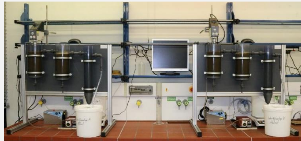
Laboratory pilot plants (activated sludge process with salt water) TU Darmstadt
